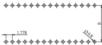
Recommended PCB Layout (PCB TOLERANCE ±0.05)
